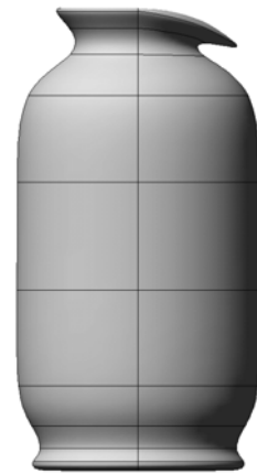
6 The revolved surface automatically updates to reflect the new curve shape. The modifications you made to the surface after revolving are preserved.
